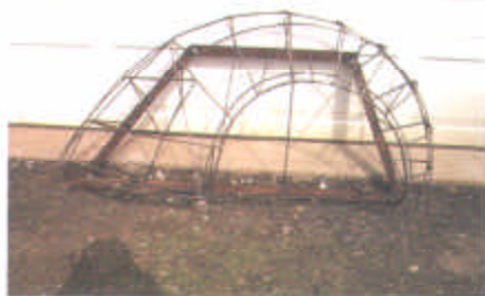
1) The wireworm is constructed of 1/4-inch steel rods, which conform closely to the inside of the original fender.
