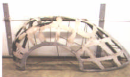
2) The wireworm is placed back into the fender after the inside of the fender has been waxed and the Bondo (or plastic filler) is applied to the steel rods.
