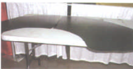
4) The flat sheetmetal has been cut 1 inch larger than the flexible shape pattern.
